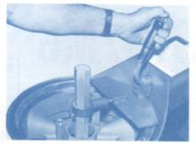
Optional equipment also includes a hold-down tool for Mags, Aluminum and Chrome Wheels, and a Top Tool for Aluminum-Mag Wheels. These tools provide secure hold down to prevent any possibility of distortion, marring or bending special type wheels.
