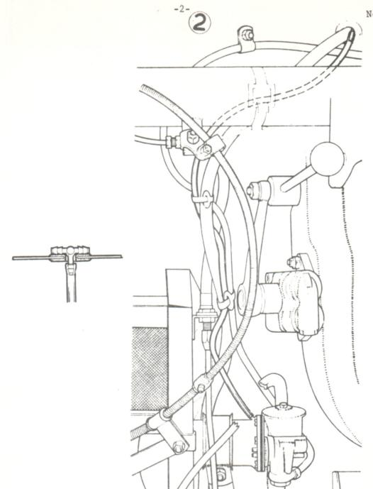
To retain the tube a plastic 'T' piece is fitted from inside the boot. The 'T' piece neck is passed through the grommet and the tube attached to the portion of the neck protruding, as shown in Fig. 1. Care must be taken that the grommet grips the 'T' piece neck and not the tube.
