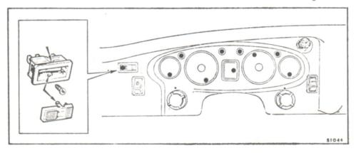
NOTE On the later 1968 Sports Cars the above switch is held into the facia panel by a wire clip. Push the clip in direction of the arrow to remove the switch.
