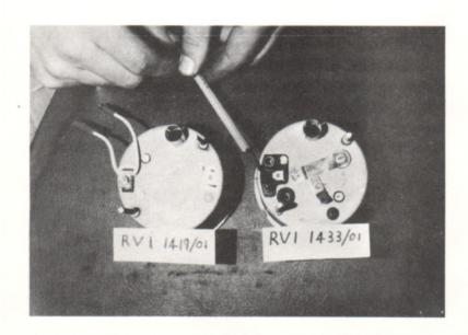
The only difference between the two is that on RVI 1433/01 the looped impulse lead is built directly into the tachometer, therefore when fitting the latest instrument simply plug the two leads from the vehicle's wiring harness directly to the terminals provided.
