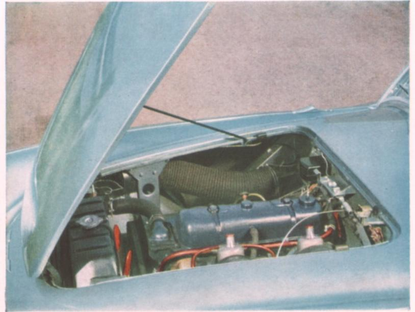
The hood is hinged along its forward edge and opens widely to give good access to the engine and ancillary components for routine maintenance.
