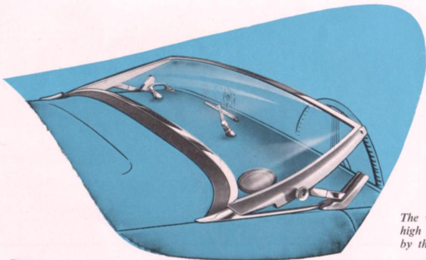
*The windshield can be neatly lowered to form a "scuttle" when high speeds are required. It is positively locked in either position by thumbscrews.*
