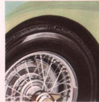
Basic models are fitted with ventilated steel disc wheels, but if continued high speed motoring, or excessive competition driving is intended, then wire-spoke wheels with "knock-on" hubs are strongly recommended. It is important that the choice should be made when ordering your car.
