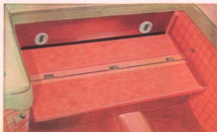
The squab of the occasional rear seats is divided and hinged in such a way that it can be folded forward to form an extended platform 19½ in. (0.49 m.) long and 36½ in. (0.93 m.) wide, when extra space for luggage is required. The surface is covered in the same hard wearing carpet as that of the floor of the car.
