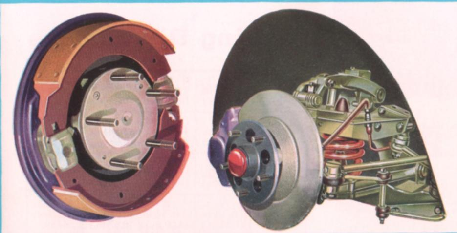
Large diameter hydraulic drum brakes are fitted on the rear wheels and with 11¼" (0.29 m.) diameter disc brakes on the front wheels, are servo-assisted to inspire confidence at the high speeds of which this car is capable.
