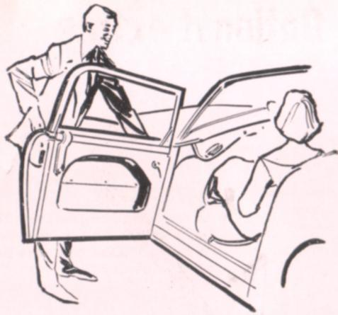
For ease of entry, forward hinged doors open wide and the lower edges lift well clear of the curb or sidewalk. Aluminum framed side screens have one fixed and one sliding plexiglass panel for ventilation or hand signaling.
