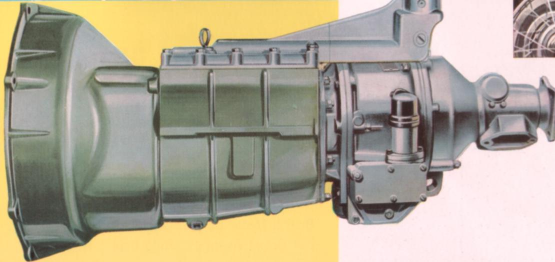
An electrically controlled overdrive (illustrated here) is fitted to the standard gearbox of the Austin Healey 3000. This is operated by a switch on the fascia and provides a high top gear ratio giving the car a fast cruising speed, while maintaining a modest fuel consumption.
