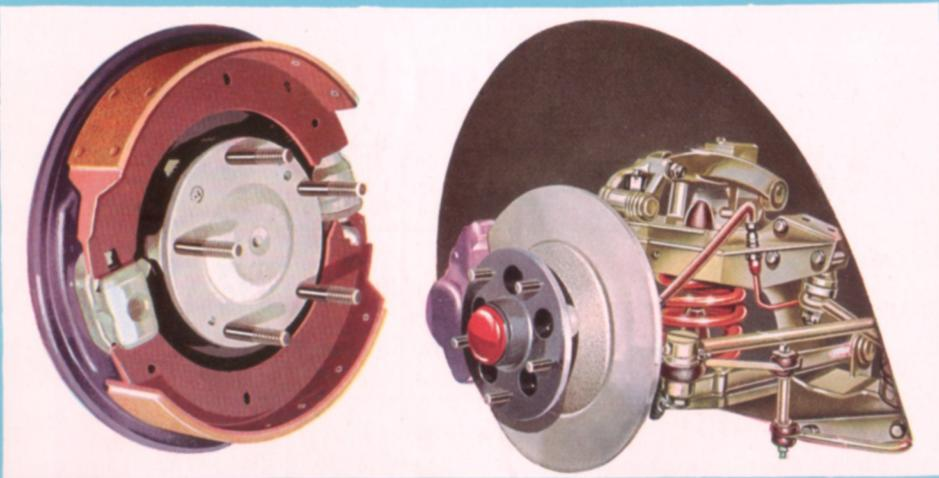
Large diameter hydraulic drum brakes are fitted on the rear wheels and with 11¼" (0.29 m.) diameter disc brakes on the front wheels, are servo-assisted to inspire confidence at the high speeds of which this car is capable.
