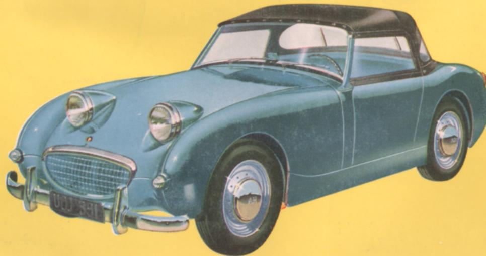
Constructionally, the accent is on safety. Independent front suspension, hydraulic shock absorbers, rack and pinion steering and an extremely low centre of gravity are features which add emphasis to the tip-tight road-holding qualities of this two-wheel-drive, integral construction is yet another feature inherent in its design . . . features have been fully developed and rigorously tested.
